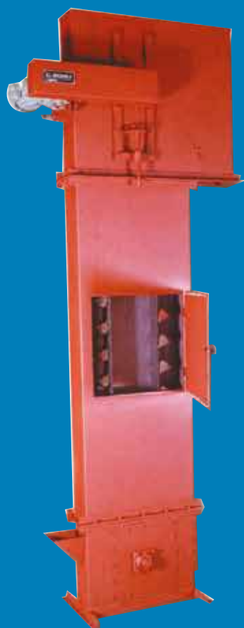
Koppelevator for stålsand.
